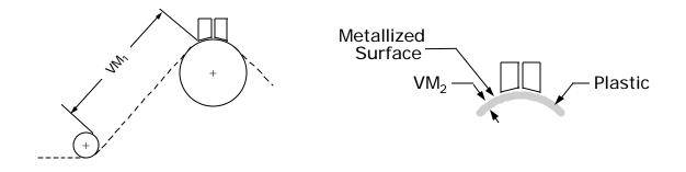
Voltage across the metallized surface between the electrode and the nearest ground roll must equal the voltage across the plastic or paper portion of the laminate.  $VM_1 = VM_2$
